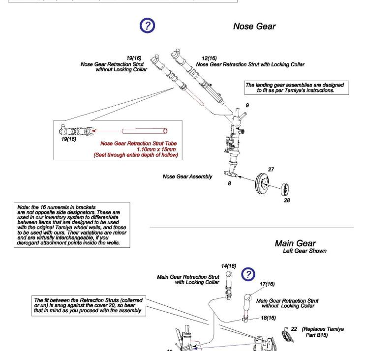
Please Note: The three blue arrows indicate the three points of contact between the gear proper (10) and the cover (20). It is essential that these points are solid connections as these will provide the necessary structural integrity for a permanently stable assembly.
